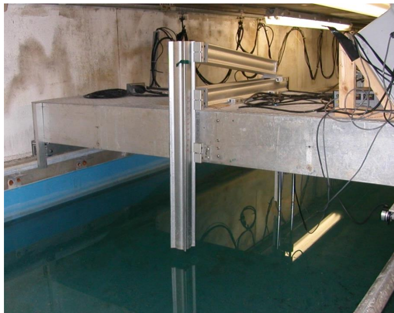
Figure 2.3 – Turbine beam mount on tow tank carriage at the University of Maine tow tank at the Aquaculture Research Center (ARC)
