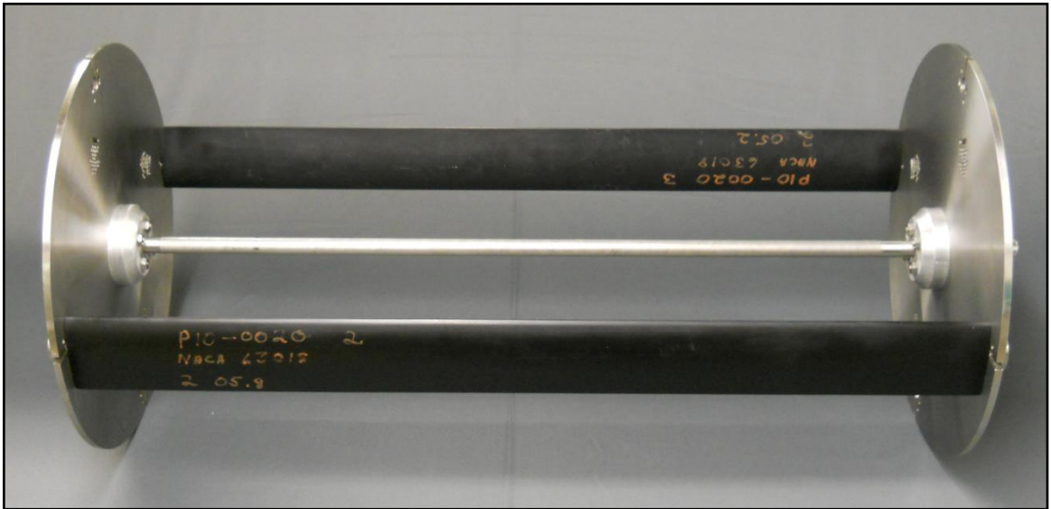
Figure A.5 – The straight bladed model Darrieus turbine rotor is shown with NACA 63 3 -018 blades installed and rod across the center.
