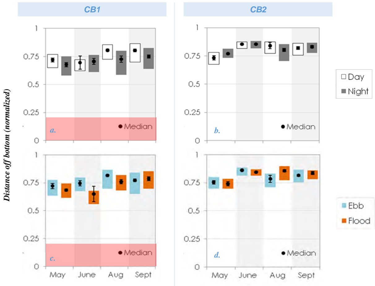
Figure 21. Mean of the median distance of individual targets off the seafloor (filled circle) and its standard error (error bars), IQR (shaded box), by site and by month. Distance off seafloor is normalized for depth changes associated with tidal cycle. Red shaded area shows region of the proposed deployment at CB1.
