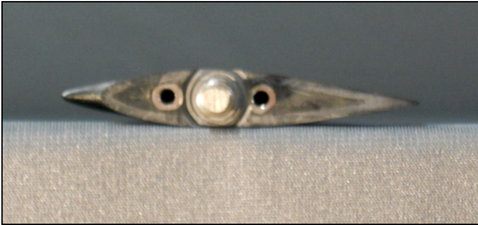
Figure 3.12 – The side view of the NACA 63 3 -018 blade is shown with tubercles added to the leading edge.
