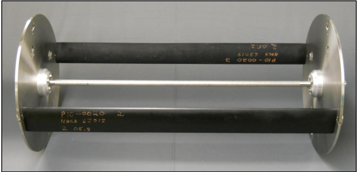
Figure 2.5. The straight bladed model Darrieus turbine rotor is shown with NACA 633-018 blades installed and rod across the center (deBree, 2012).
