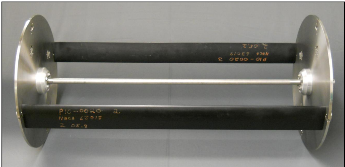
Figure 1.3 – The straight bladed model Darrieus turbine rotor is shown with NACA 63 3 -018 blades installed and rod across the center.
