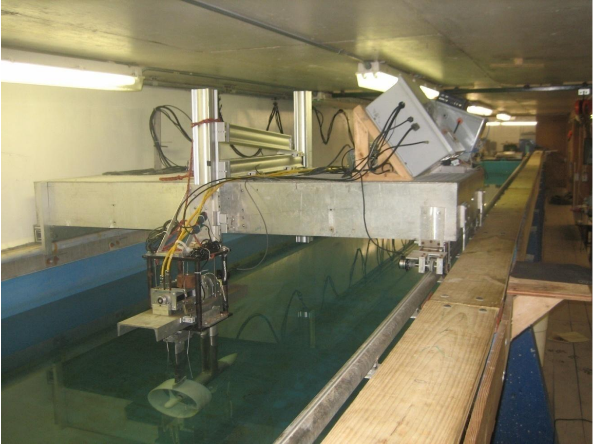
Figure 3.2 UMaine tow tank with ducted turbine installed ready for testing.
