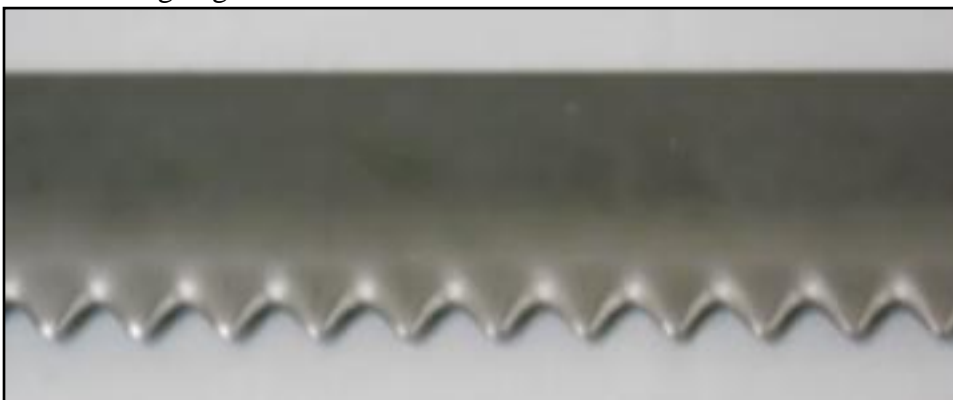
Figure 3.13 – The top view of the NACA 63 3 -018 blade profile is shown with tubercles added to the leading edge.
