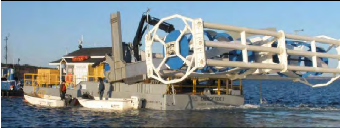
Figure 3.2. Research platform. ORPC's Energy Tide II, showing test turbine in raised position.
