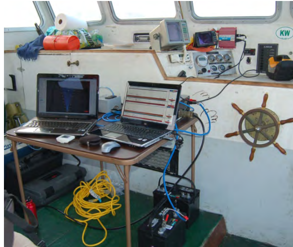
Figure 6. Arrangement of DIDSON control computer, SIMRAD control computer and transceiver unit behind (right), and storage batteries for operation of the DIDSON and SIMRAD transceivers.
