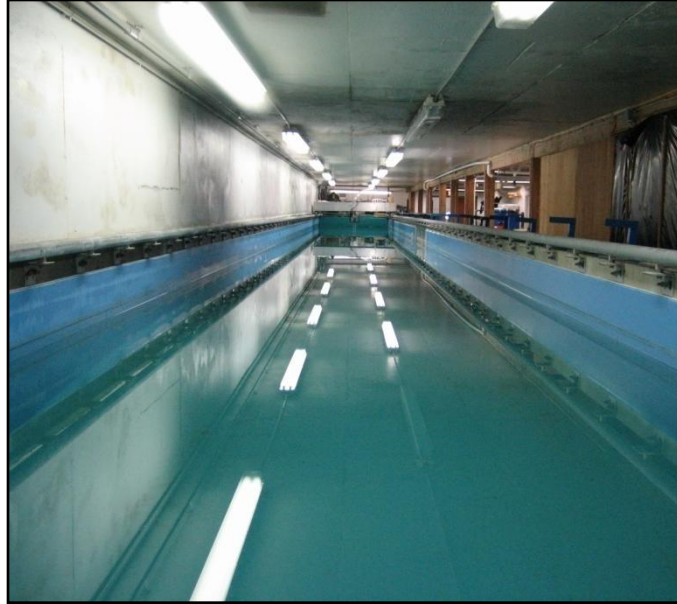
Figure 3.1 – The University of Maine tow tank is shown with rails and carriage in the distance.
