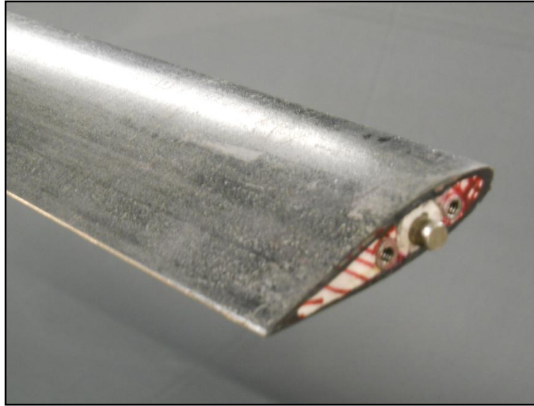
Figure 3.10 – The NACA 63 3 -018 carbon fiber turbine blade is shown with locating rod and tapped mounting holes.
