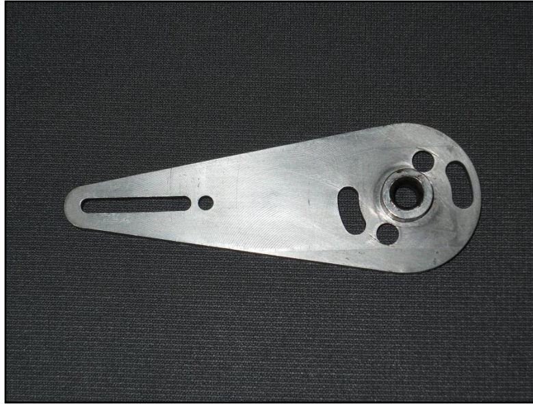
Figure 3.6 – The center hole in the angle indicator accepts the blade mounting rod. The center hole protrudes out of the page, and when installed in the indicator mounting hole, it extends all the way through the end plate. This section transfers the blade loads from the blade to the end plate.
