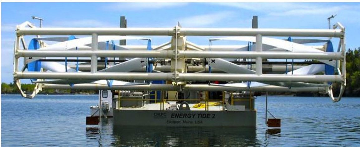
Figure 1.2 - A cross-flow hydrokinetic turbine is shown above water (Image Source: http://www.orpc.co/newsevents_photogalleryDetails.aspx?Aid=i1%2bgAhwr%2boY%3d ).
