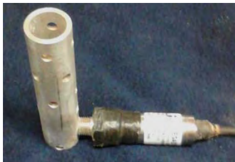
Figure 3.12 Pressure transducer and flow shroud configuration to measure the surface elevation on the floor of the tow tank.
