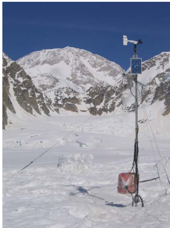
Figure 2. Base camp AWS on May 6, 2009 after downloading data and elevating the instruments for a second year of data collection. Three additional guy wires were attached for added stability when the snowpack melts during the summer.
