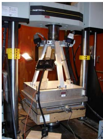
Figure 2. Hydromat test system with digital image correlation system
