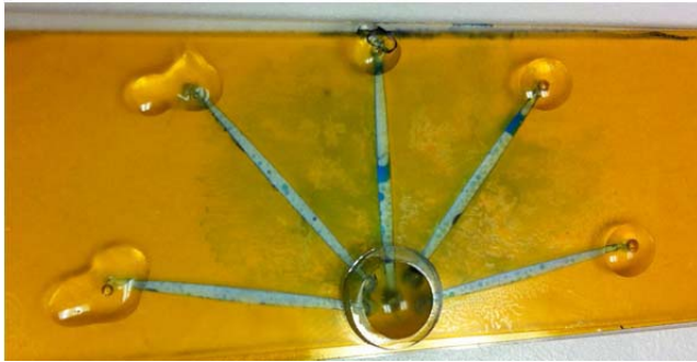
Figure 1. De-lamination of fluid (blue) occurs at higher temperatures in stationary chambers unless heating and a spark-treatment occur during fabrication.
