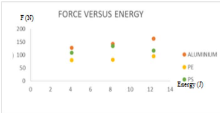
Figure 1-10 – Drop impact tests, three different impact heights were used which are 0.2, 0.4 and 0.6 m, [21].
