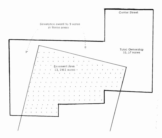
It is sometimes helpful to produce an illustration or diagram to explain why a severance damage can occur in a case such as this. Exhibit 8 has been reproduced showing the long, triangular and irregular shaped fringe areas located to the north and west of the easement area taken. It takes little imagination to see why any reduction in the nature of the use of the 13.1961 acres would also substantially apply to those 9 acres.
