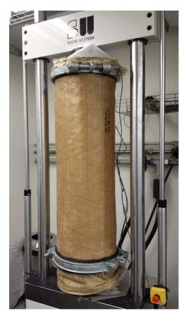
Figure 3-2. Photo of a specimen installed in the tension-torsion test machine.
