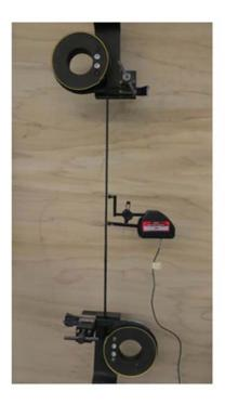
Figure 2-7. Photo of instrumented cord in tension test fixtures.
