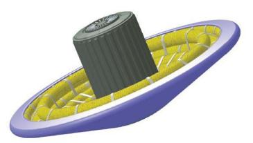
Figure 1-2. Conceptual rendering of HIAD with payload (gray) and flexible thermal protection system (purple) (Young, 2017).
