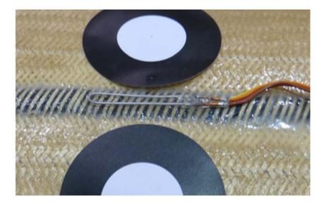
Figure 2-10. Photo of liquid metal strain gage courtesy of Nino Piazza, NASA Armstrong.
