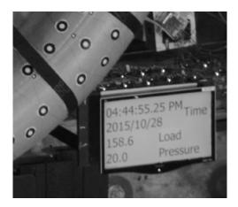
Figure 5-7. Photograph of example live information displayed during a torus test: time, date, total load (lbf), and pressure (psi).
