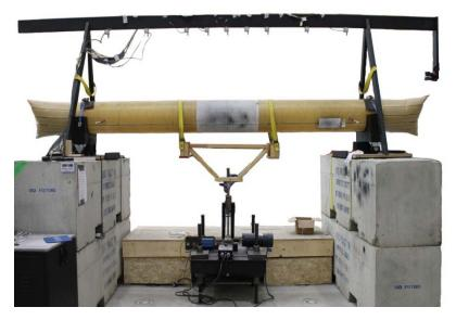
Figure 4-2. Photo of bending test setup.
