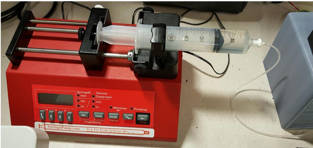
Figure 6: New Era NE-1000X bidirectional programmable syringe pump. With fully programmable and stand-alone capabilities, the pump can be programmed for up to 41 pumping phases that change pumping rates, set dispensing volumes, insert pauses, control and respond to external signals. It has a dispensing accuracy of \pm 1\% .
