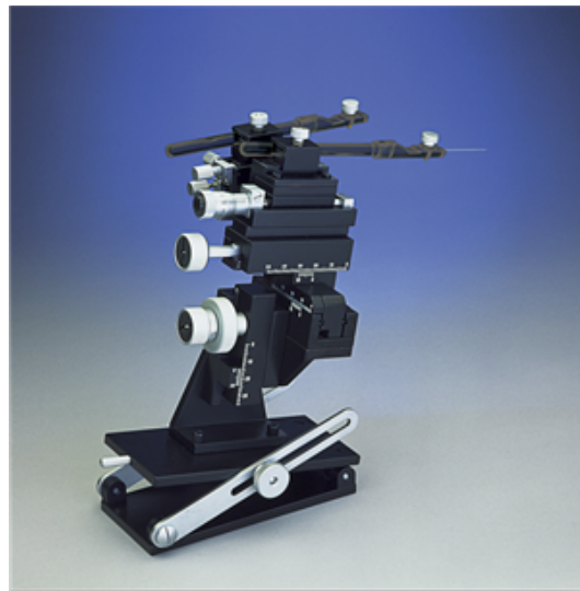
Figure 2: A typical micromanipulator for manual injection needle operation in all three axes (x, y and z). It allows for coarse adjustment readings with an accuracy of 100 micrometers. Warner Instruments, Model MM-33, Hamden CT.
