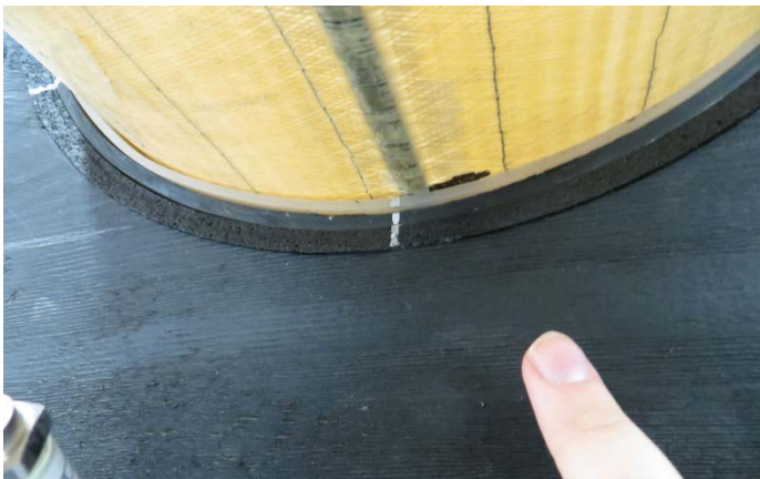
Figure 4.10. Cord misalignment during straight tube four-point bending test.
