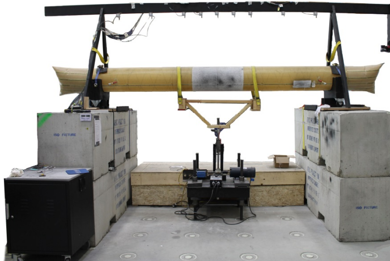
Figure 4.1. Straight tube four-point bend test configuration.
