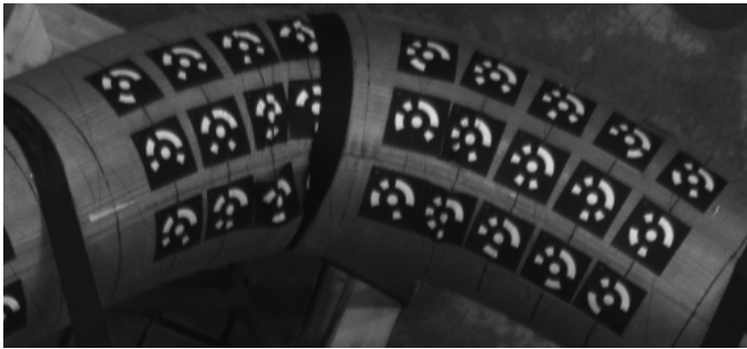
Figure 4.18. Out-of-plane strap/torus penetration, before and after initial wrinkling (Whitney 2016).
