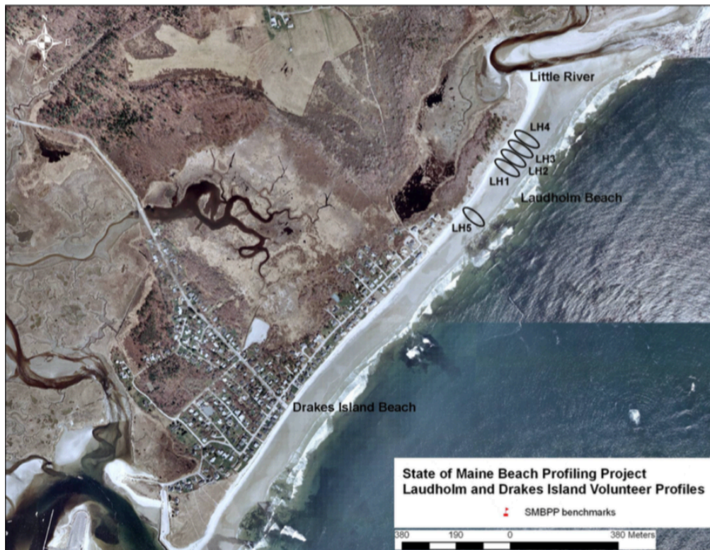
Figure 5. A black circle marks the general location and area for each profile location at Laudholm Beach. From the northeast (Little River) to the southwest (Drakes Island Beach) the profiles are as follows: LH04, LH03, LH02, LH01, and LH05. All profiles are unarmored (Slovinsky & Dickson, 2007).
