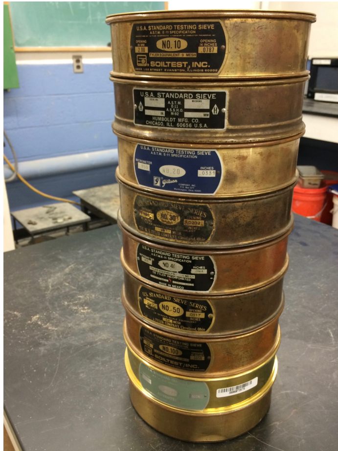
Figure 22. Sieve stack used for grain size distribution testing. Sieves are organized by opening size, descending from largest at the top (#10) to smallest at the bottom (#200) (DeVoe, 2016g).
