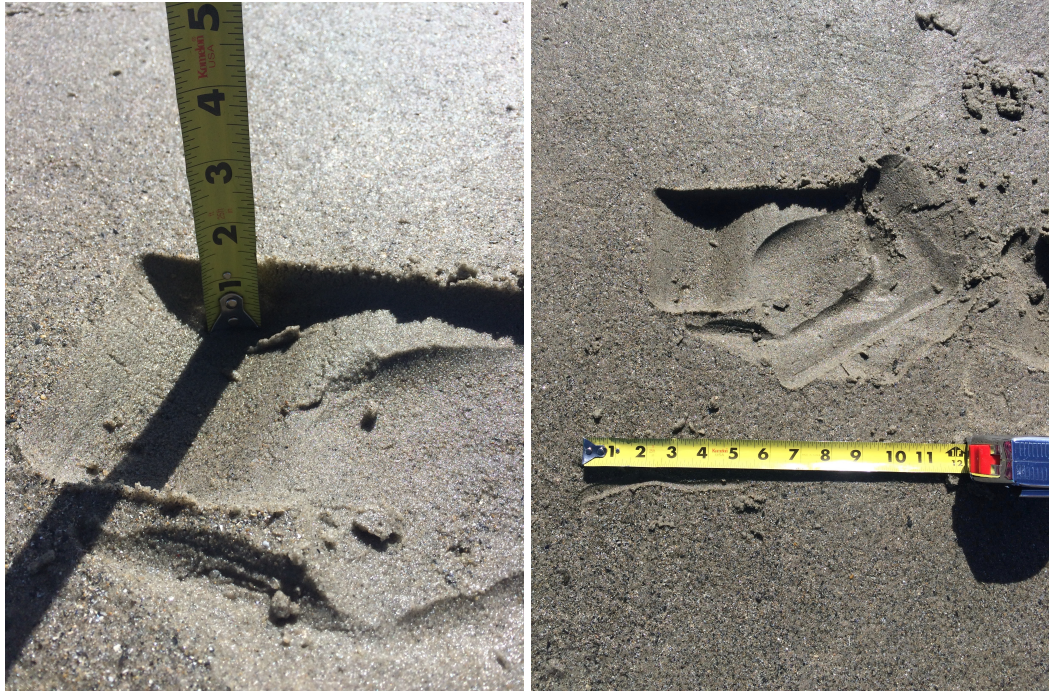
Figure 20. Typical sample collection site dimensions – 2 inches in depth, left, and 1 foot square, right. Samples were obtained from shallow collection sites to minimize the impact of non-surficial materials upon sieve results (DeVoe, 2016b).
