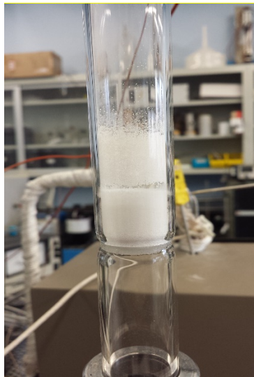
Figure 5: Image of the reactor without the heat tape so that the particle bed fluidization could be visualized.
