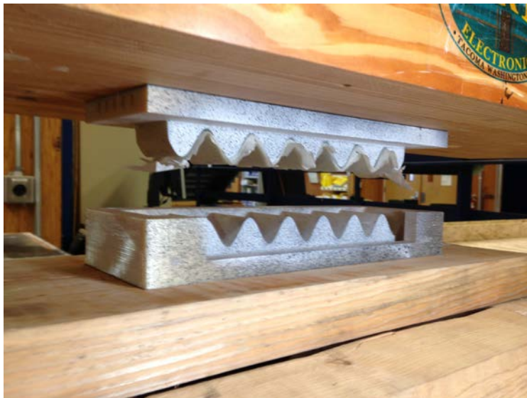
Figure 6.16: The formed part stuck to the male mold after pulling the mold to the top.
