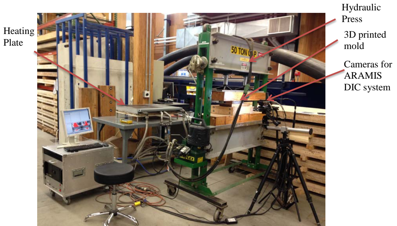
Figure 6.15: Setup for experimental verification of the finite element model.
