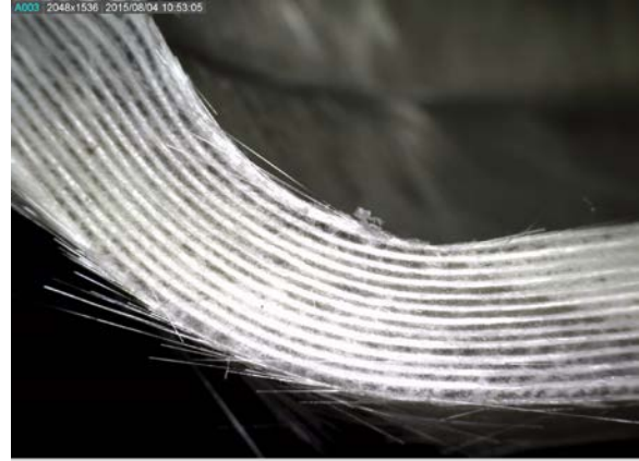
Figure 2.15: Cross-section of the formed part along curved section.
