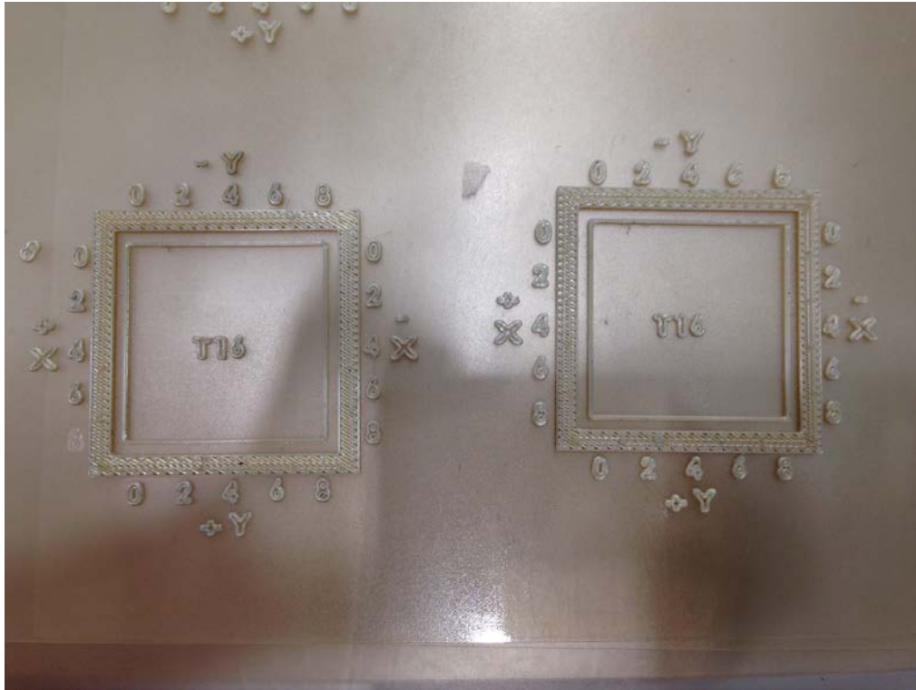
Figure 2.7: Calibration Squares printed during calibration of Stratasys Fortus 900 mc.
