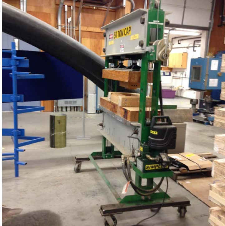
Figure 2.10: The press with wooden box frame, mold and silicone foam rubber.
