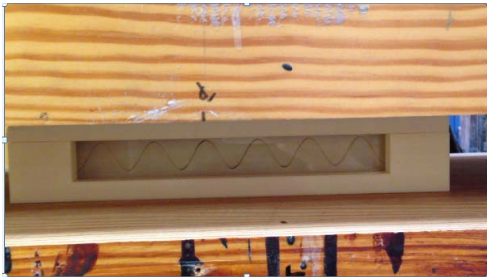
Figure 6.6: Bending reduced due to reinforcements in male mold.
