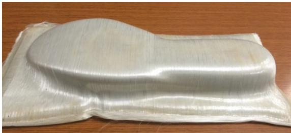
Figure 2.12: Bottom side of formed part with 25 layers of prepreg tapes.
