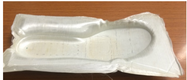
Figure 2.13: Top side of formed part with 25 layers of prepreg tapes.
