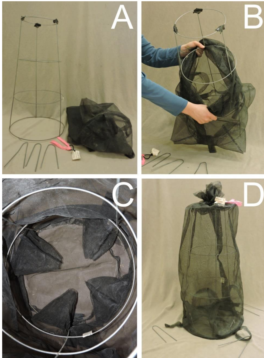
Figure 14. Assembly of traps in the field. (A) The components of the trap: altered tomato cage, fiberglass screening sack, stakes, and hair elastic equipped with flagging tape and a tag. (B) Inserting the frame into the sack is made easier by pulling the funnels inside-out so they do not get caught on the bars of the cage. (C) A view looking down into the trap after inverting the funnels. (D) The top of the sack is gathered and secured with the hair elastic, and the trap is stacked to the substrate through straps at the bottom of the sack.
