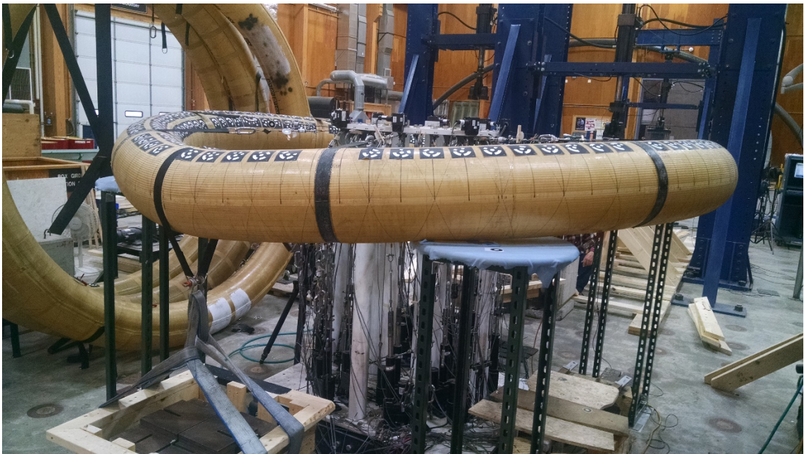
Figure 90: 2.1kN Out-of-plane Test Just Prior to Failure
