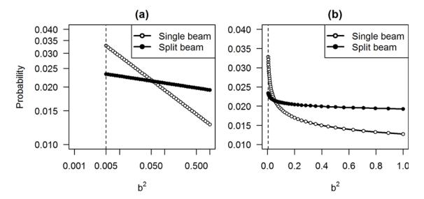
Fig 2.6 Beam pattern probability density function.  $w_T(b)$  shown for the 200 kHz single and split beam echosounders, with (a) logarithmic and (b) linear axes. Vertical line indicates minimum intensity included in analyses (0.005). The beam intensity shown is squared, as sound is affected by the beam pattern twice as it travels to and from a reflective object.
