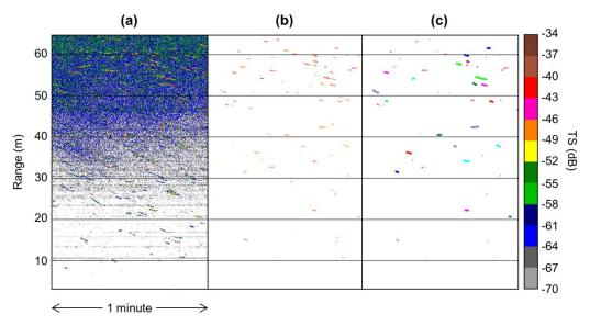
**Fig 3.4 Acoustic data processing example.** (a) Raw target strength data (scale in dB to right) showing multiple fish tracks and background noise. (b) Target strength data with noise removed and -50 dB TS threshold applied. (c) Single targets detected from cleaned target strength data with fish tracks (colored lines) overlaid.
