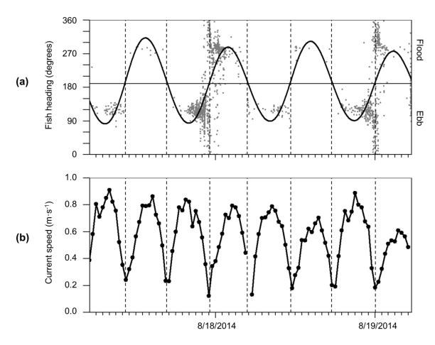
**Fig 3.5 Fish heading and current velocity.** Data **were** collected at the TidGen® site in March 2013. (a) Individual fish heading (gray points) shown with fitted tidal model (solid line) and its midline (horizontal line), which were used to calculate times of slack tide (vertical dashed lines). (b) Current speed collected concurrently by an ADCP at the same site, with same times of slack tide as shown in (a).
