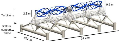
Fig 2.1 Ocean Renewable Power Company's TidGen® Power System. Turbine image provided by ORPC.
