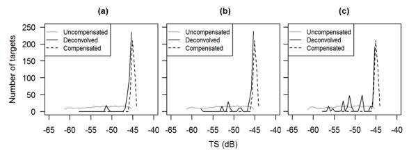
**Fig 2.4 Results of deconvolution of sphere TS.** Three different smoothing window lengths were used: (a) 0.7, (b) 0.5, and (c) 0.3 times the length of the PDF.
