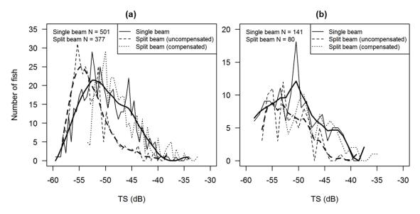
**Fig 2.7 Distribution of TS data from single beam and split beam echosounders.** (a) August 2012 and (b) March 2013. Data were divided into 20 backscatter bins per decade in August, and 10 per decade in March. The number of fish in each sample (N) shown in upper right. Thick lines indicate smoothed TS distributions (using a window size of 0.5 times the PDF length) which were used in deconvolution.
