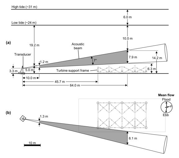
**Fig 3.2 Echosounder setup in Cobscook Bay, Maine.** The bottom support frame of Ocean Renewable Power Company's TidGen® device was present during data collection. The gray area indicates the sampled volume used in this study. TidGen® schematic provided by Ocean Renewable Power Company
