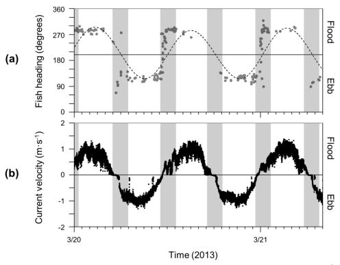
**Fig 1.6 Fish heading and current velocity.** Example from data collected at the TidGen® site in March 2013. (a) Individual fish heading (gray points) shown with fitted tidal model (dashed line) used to calculate times of slack tide (gray areas). (b) Current velocity collected concurrently by a bottom-mounted ADCP at the same site.
