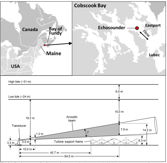
**Fig 4.1 Study area and echosounder setup.** In lower panel, tidal current moves out of page during the ebb tide and into the page during the flood tide. Figure components from Chapter 3.
