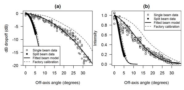
**Fig 2.5 Results of echosounder calibrations.** Beam pattern shown as (a) dB dropoff and (b) intensity at a range of off-axis angles. Points are calibration data, the thick lines are models fit to each echosounder's calibration data, and the dashed lines are the factory-specified beam patterns of each transducer.
