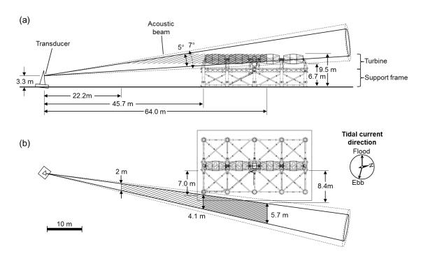
**Fig 1.3 Echosounder and TidGen® setup.** (a) Side view; (b) view from above. The "turbine" zone of the sampled volume is indicated by the darker hatched region, and the "beside" zone by the lighter hatched region. The median current direction for each tidal stage, estimated from fish heading data (see text), is shown at right in (b).
