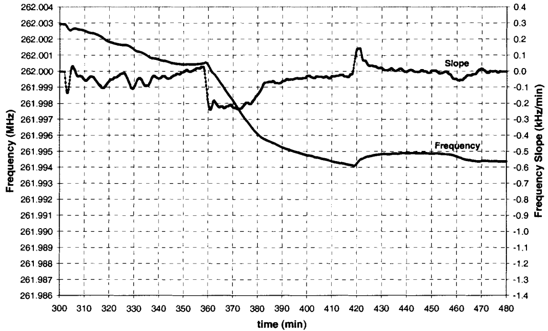
Figure A.16 500 Å gold film exposed to 40 ppb mercury.
