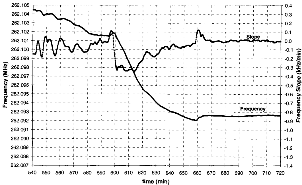
Figure A.22 300 Å gold film exposed to 60 ppb mercury.
