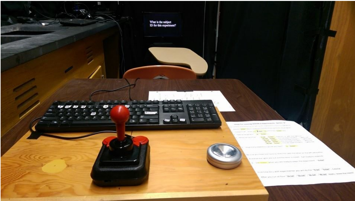
Figure 2.2 View of the experimental station from the subjects prospective. The computer screen is 10' away from the subject. The keyboard is used for setting up the trials. The jystick is used to select where the subject thinks the break occurs.
