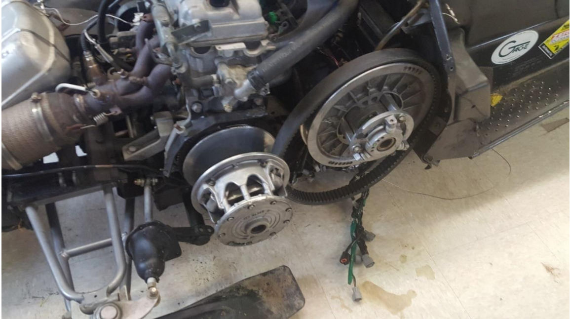
Figure 18: 2004 Arctic Cat 4-Stroke CVT System
