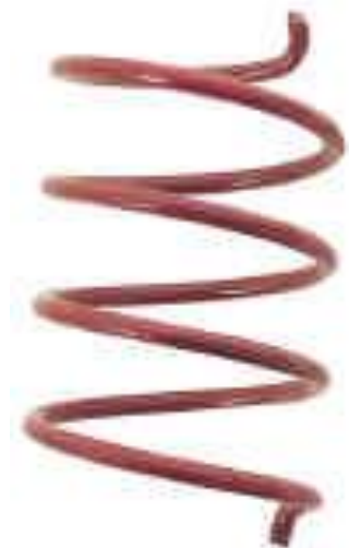
Figure 6: Arctic Cat Pretension Spring [7]
