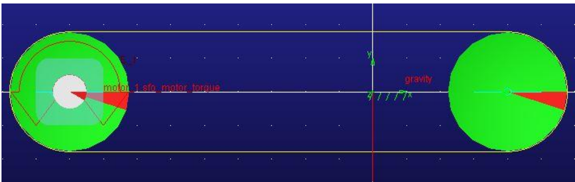
Figure 26: Side View of a CVT in a 1:1 mid-ratio
