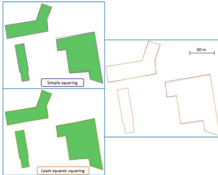
Figure 9: Extract of squared buildings with more complex shapes from Würzburg area, initial shapes in green.
