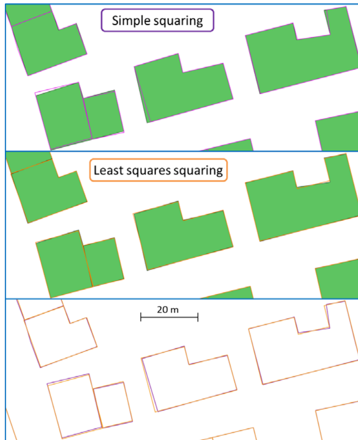
Figure 8: Extract of squared buildings with simple shapes from Würzburg area, initial shapes in green.
