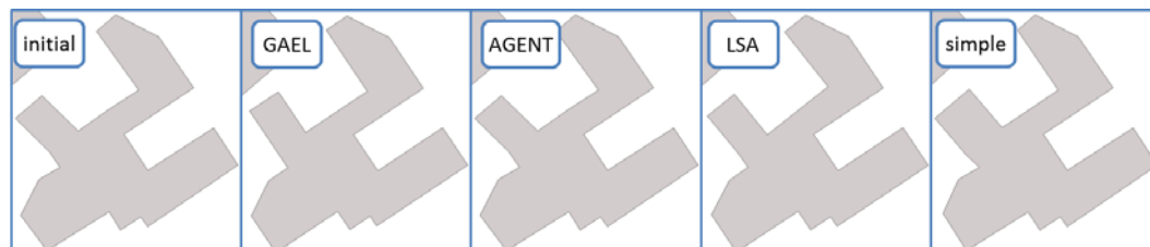
Figure 18: Comparison of all squaring method for a given complex building footprint, LSA stands for Least Squares Adjustment.
