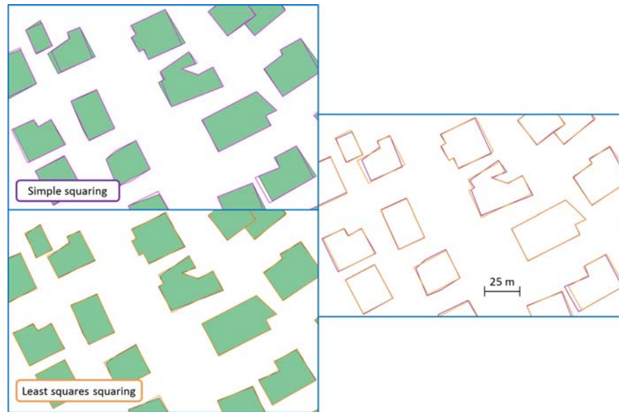
Figure 10: Extract of squared buildings with simple shapes from IGN reference dataset, initial shapes in green.
