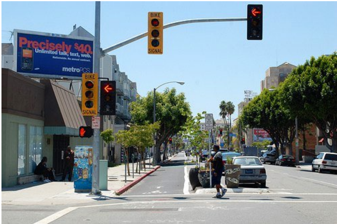
Figure 3.7. Bike Signals at Intersection (LADOT Bike Blog, 2011)
