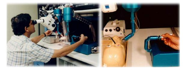
Figure 1-21: JPL Robot-Assisted Micro-Surgery (RAMS) system.
