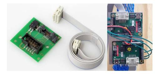
Figure 4-9: Motor/encoder connector (left) and DC brushed controllers (V) & (VI) wired to the system (right).
