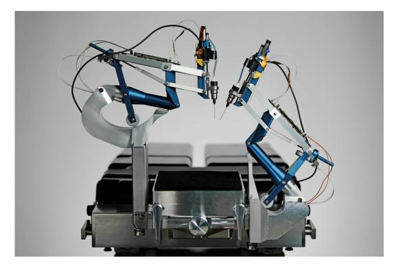
Figure 1-17: Eye-RHAS, eye robot for haptically assisted surgery (Meenink 2011)
