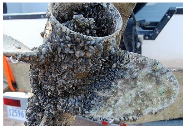
Figure 5: Zebra mussels attached to a boat rudder removed from Lake Austin, Texas (Photo courtesy of Colorado River Alliance)
