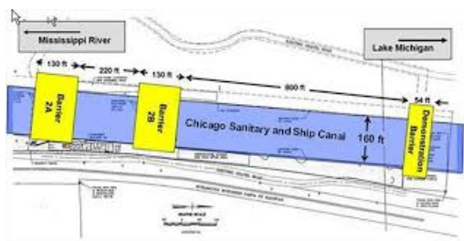
Figure 4- Right; Diagram displaying the 3 electric barriers and their orientation to Lake Michigan and the Mississippi River. Figure from: www.lrc.usace.army.mil/Missions/Civil-Works-Projects/ANS-Portal/Barrier/ .
