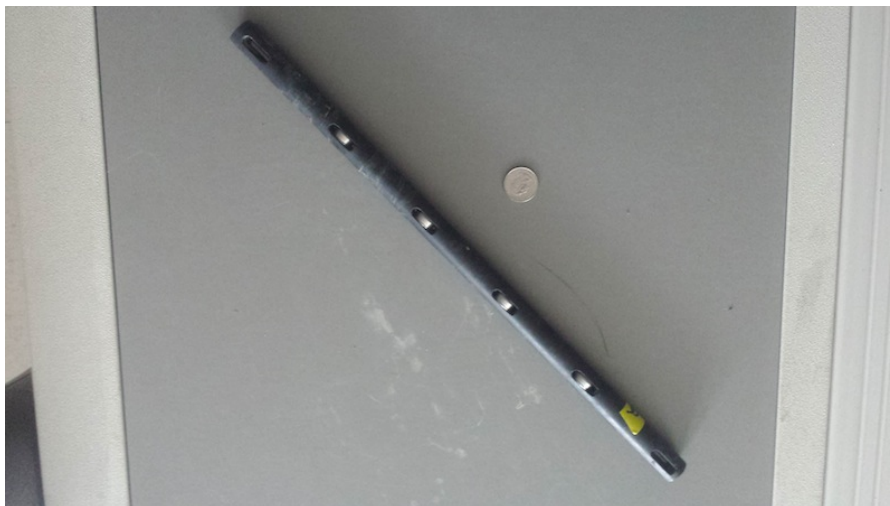
Figure 3: iButton and Deployment Stick. iButtons housed in the machined plastic rod. A U.S. quarter (2.42 cm diameter) is shown for scale.
