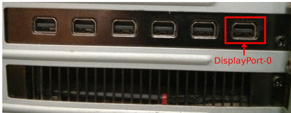
Figure 2.6: ATI Radeon HD 5870 Port Layout
