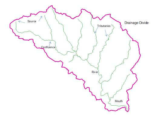
Figure 4.4 Parts of a Stream Network
