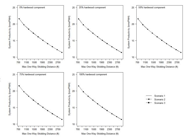
**Figure 1.7:** System productivity of a grapple skidder and stroke delimber system based on various hardwood components and an average bunch spacing of 48 ft and a removal intensity of 40 tons per acre. The productivity of all three scenarios is similar and thus the individual lines are overlaying each other.
