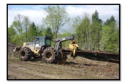
**Figure 1.1:** A grapple skidder generally transports several trees in a bunch from the forest to the roadside where the whole trees get processed by a stroke delimber.
