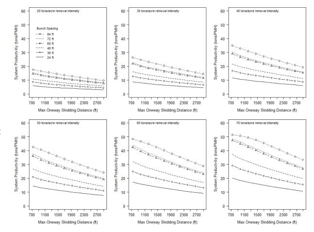
**Figure 1.5:** Grapple skidder and stroke delimber system productivity based on removal intensity and bunch spacing with a 50% hardwood component when using the baseline scenario (Scenario 1). PMH = productive machine hours.
