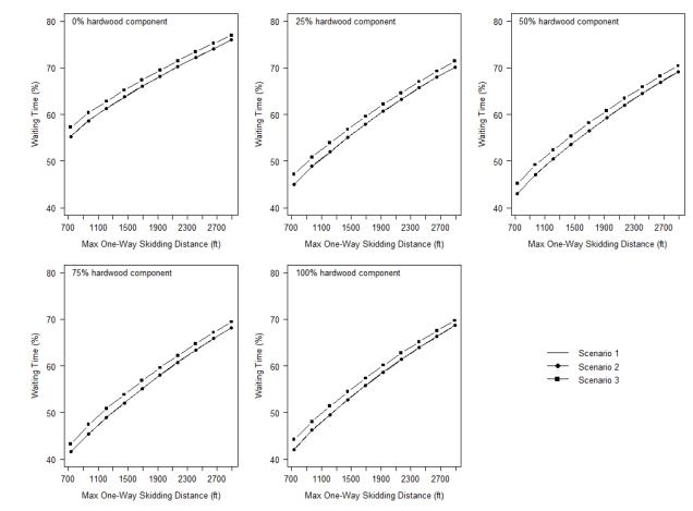
**Figure 1.6:** Stroke delimber waiting time based on various hardwood components and an average bunch spacing of 48 ft and a removal intensity of 40 tons per acre. No difference was found between Scenario 1 and Scenario 2 and both lines are approximately on top of each other.
