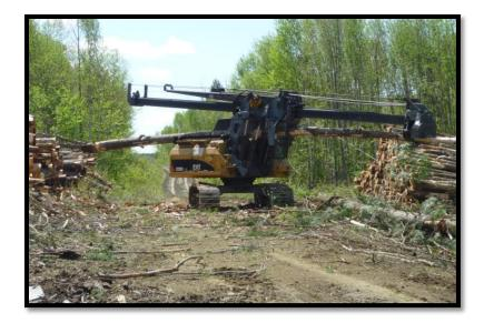
**Figure 1.2:** A stroke delimber generally processes one tree at a time by cutting of branches and the top above a specific merchantable diameter.
