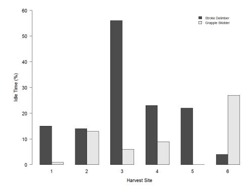
**Figure 2.1:** Stroke delimber and grapple skidder idle times as observed during a study by Hiesl (2013).
