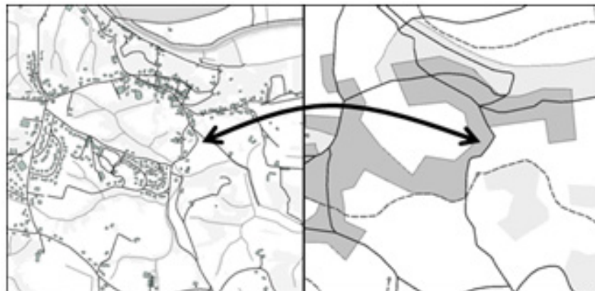
Figure 1: The matching problem. A pair of identical features in two different representations of the same world.
