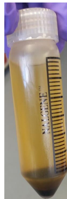
Figure 4: Iron Nanoparticles Separated by Ethanol via Centrifugation
