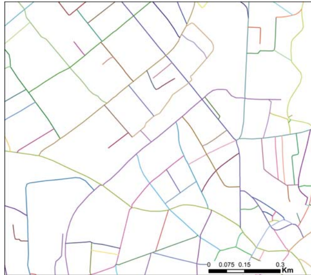
Figure 9: The resulting strokes exhibit a much better continuity after the roundabouts have been identified and collapsed. (Data © swisstopo)
