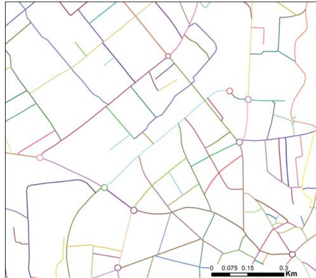
Figure 7: The roundabout problem: they disrupt important strokes and impede their continuity. It is also important to note that the roundabouts form exactly one stroke in most cases, which is a property exploited in the detection algorithm. (Data © swisstopo)
