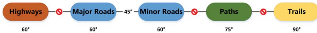
Figure 11: This diagram shows the five primary road class groups, which were created based on the width-based road classes used in the TLM3D dataset. Each group uses a separate angle threshold in the stroke building process. The algorithm can be adapted in order to either constrain or relax the conditions under which strokes are generated.
