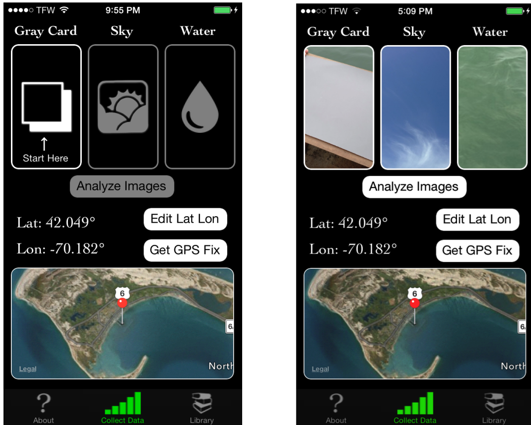
Figure 5.2. HydroColor data collection view. This display is meant to acquire and display GPS information and to begin walking users through image collection. The left and right screenshots show the data collection view before and after image collection.
