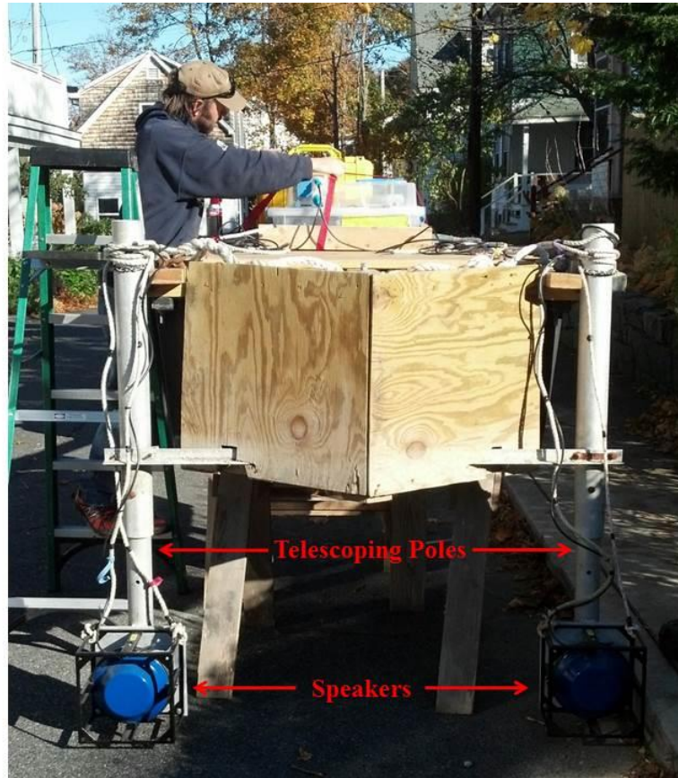
Figure C.1. Front View of Attachment Platform. All acoustic and electronic components are attached. Poles allow speaker centers to be deployed at multiple depths and angles, approximating variations in test ship hull design.
