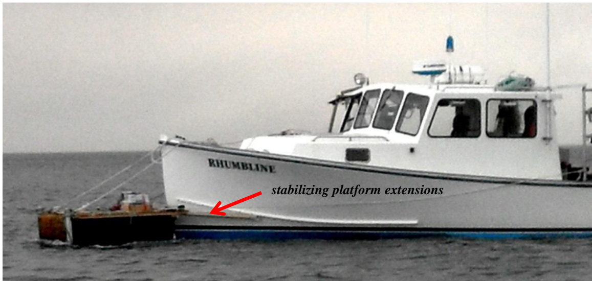
Figure 4.3 Prototype Attached to Test Ship Rhumbline Underway at 4.2 Knots. The adjustable platform extensions are located below the rub rails, providing downward force on the rear of the platform thereby increasing platform stability.
