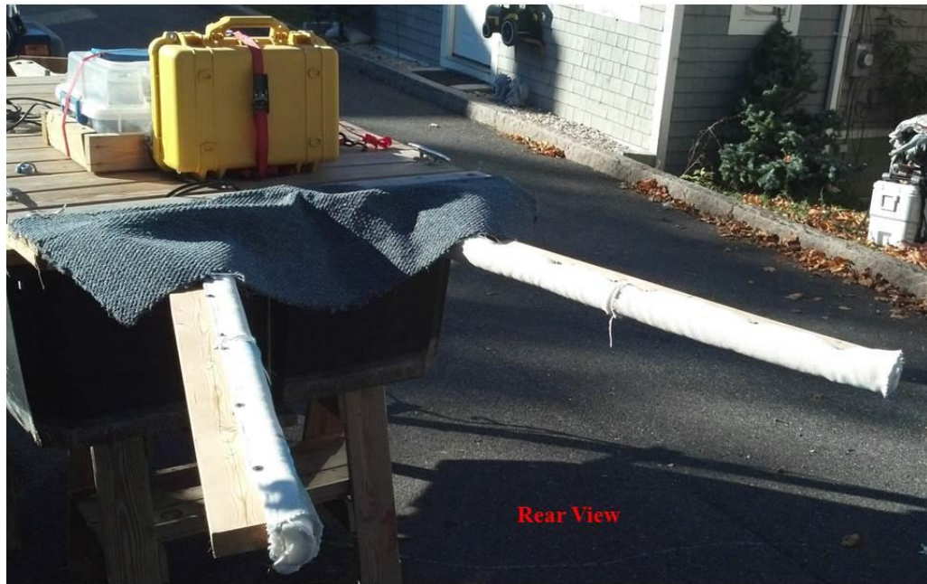
Figure C.5. Close-Up of Platform Extensions. Platform extensions are padded and adjustable to the width of each test ship's bow. An additional notch is cut into the back of the platform, beneath the carpet padding.
