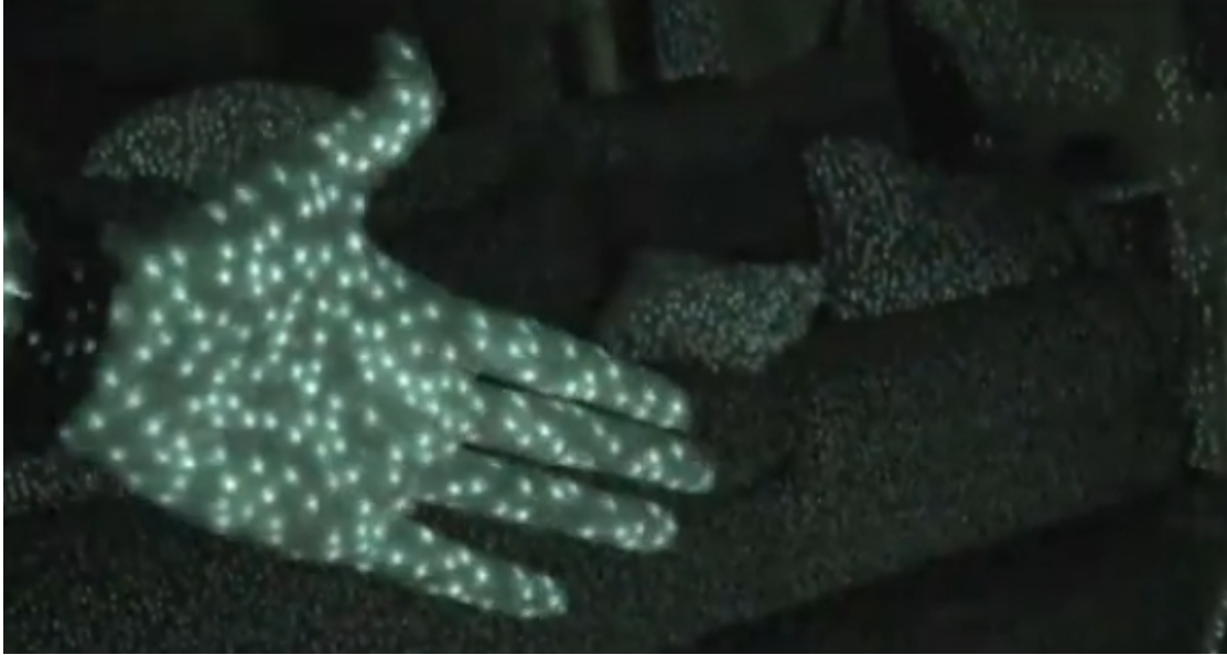
Figure 6. Infrared image of the Kinect in action
