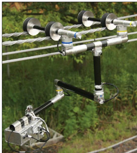
Figure 13: HIBOT's EXPLINER (15, HIBOT)
