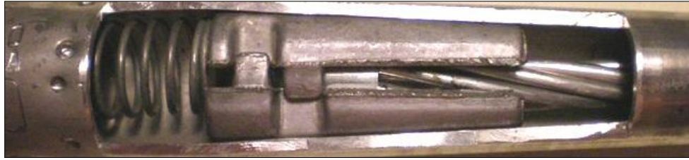
Figure 5: Automatic Wedge Splice
