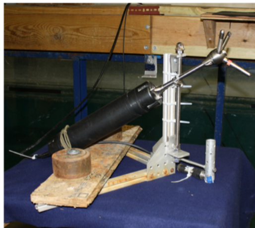
Figure 3.14 ADV and pressure transducer with flow shroud mounted to the adjustable floor tripod.
