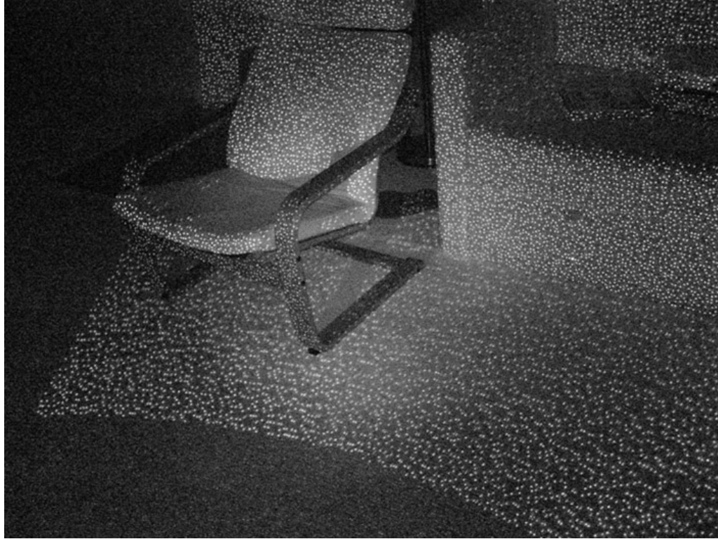
Figure 2.2. The infrared pattern projected by the Kinect sensor
