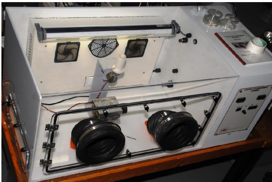
Figure 5.1 – Environment controlled chamber with dipping apparatus
