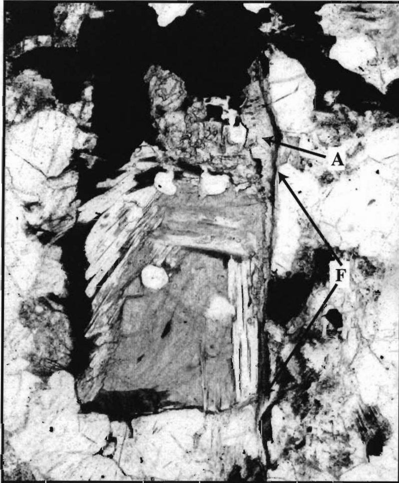
Figure 2.8 Photomicrograph of pseudomorphed andalusite. Andalusite (A) partially pseudomorphed by coarse muscovite and a fine-grained mat of intergrown chlorite and muscovite. Fibrolite (F) rims a portion of the porphyroblast.
