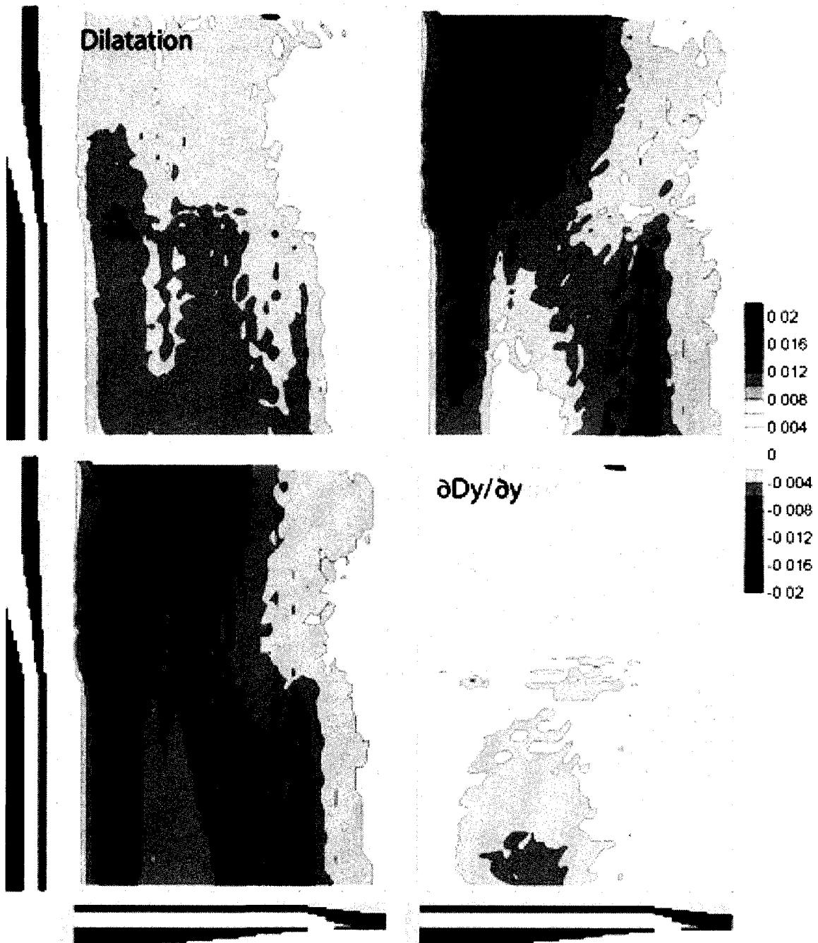
Figure 6.14. Model 3 dilatation, pure shear, \partial D_x/\partial x , and \partial D_y/\partial y .
