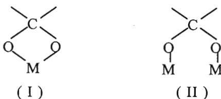
Scheme 5.1 (I) bidentate chelating and (II) bidentate bridging structures on metal oxide surfaces
