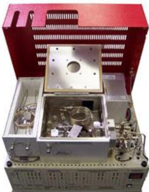
Figure A-1: A typical SRI GC multiple gas analyzer with sulfur detector #2
