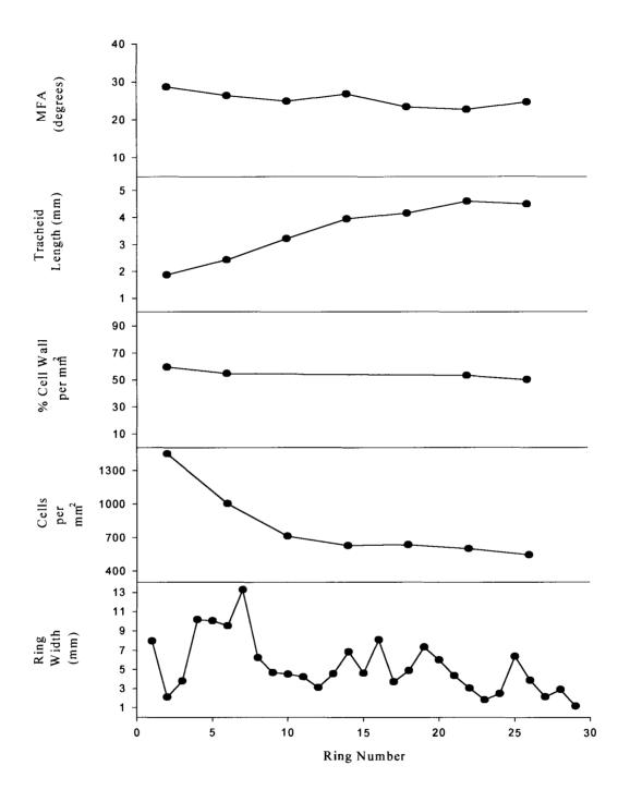
Figure 2.1 Tracheid dimensions of *Metasequoia glyptostroboides* (PNJ tree) versus ring number from pith. (MFA and tracheid length adapted from Jagels et al., in prep)
