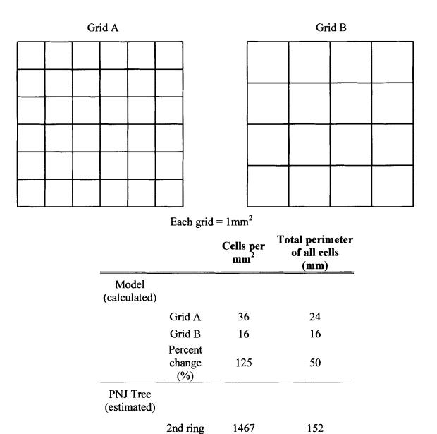
Figure 2.4. Changes in total perimeter of all cells per  $mm^2$  as a function of cell size in transverse sections -- theoretical model and estimated values from the PNJ tree.
