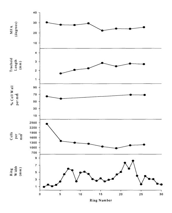
Figure 2.2 Tracheid dimensions of *Metasequoia glyptostroboides* (JPC tree) versus ring number from pith. (MFA and tracheid length adapted from Jagels et al. in prep)
