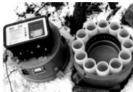
Figure 6. ISCO autosampler used at PRIMENet stream sites. The datalogger (left) locks into place above the sample bottles.
