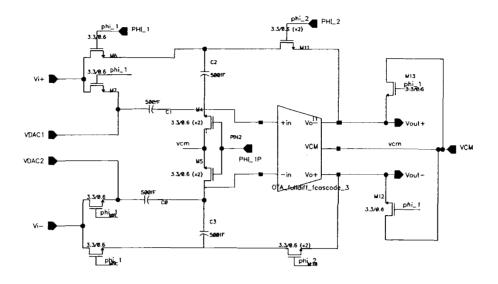
Figure 4.6: S/H and gain portions of the stage.
