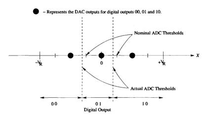
Figure 2.8: Sub-DAC outputs in the 1.5 bits/stage architecture.
