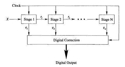
Figure 2.1: Generic Pipeline ADC block diagram.
