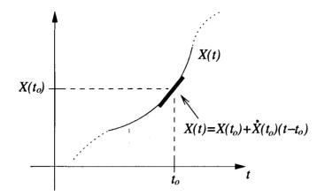
Figure 2.15: Time varying S/H input signal.
