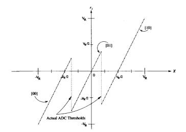
Figure 2.12: Error characteristics for a single stage with actual thresholds.
