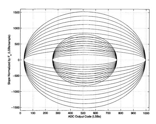
Figure 3.2: Calibration trajectories in the code/slope space.
