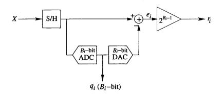
Figure 2.2: Generic stage block diagram.
