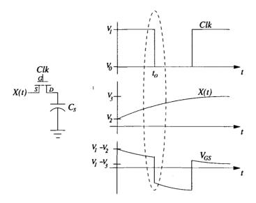
Figure 2.16: Model of S/H circuit.
