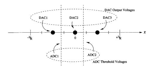
Figure 2.18: Locations of parameters for simulated ADC.
