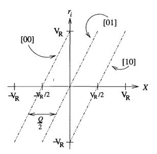
Figure 2.10: Residual characteristics for 1.5 bits/stage.
