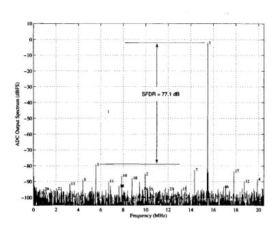
Figure 2.13: Spectral plot of THS1240 ADC with  $F_t = 15.5$  MHz.
