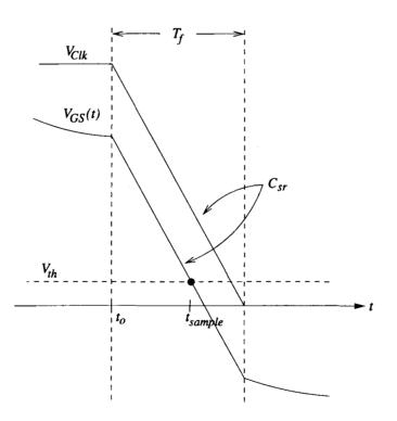
Figure 2.17: Special case in S/H circuit.
