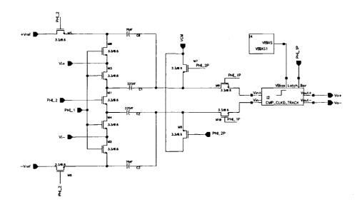
Figure 4.5: Differential Comparator implementation.
