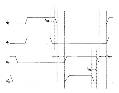
Figure 4.3: 2-Phase Non-Overlapping Clock Timing.
