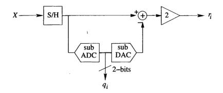
Figure 2.7: Block diagram of a single stage (1.5 bits/stage).
