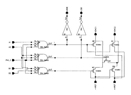
Figure 4.7: Sub-DAC circuit implementation.
