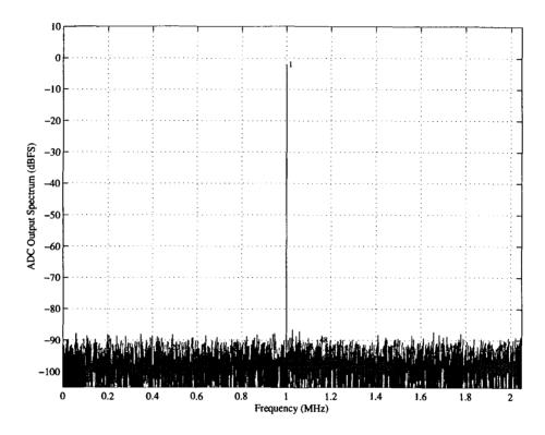
Figure 2.14: Simulated 10-bit Pipeline (Ideal) with  $F_t = 1$  MHz.
