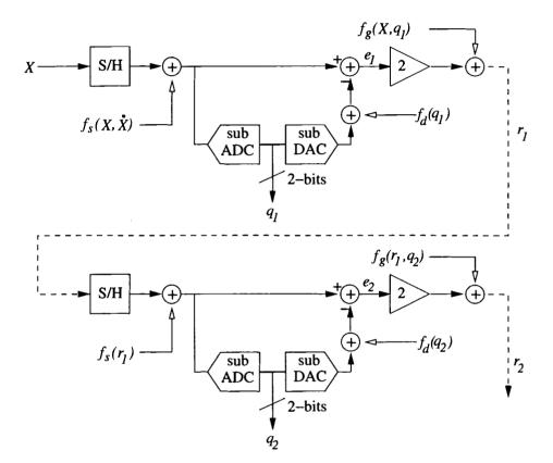
Figure 3.1: First and second stage block diagram with error models.
