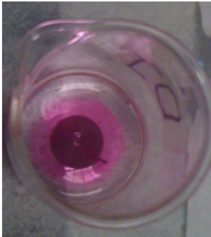
Figure 5.5 Photograph of MSCAT sensor with the E. coli antibody film after the introduction of Amplex Red.
