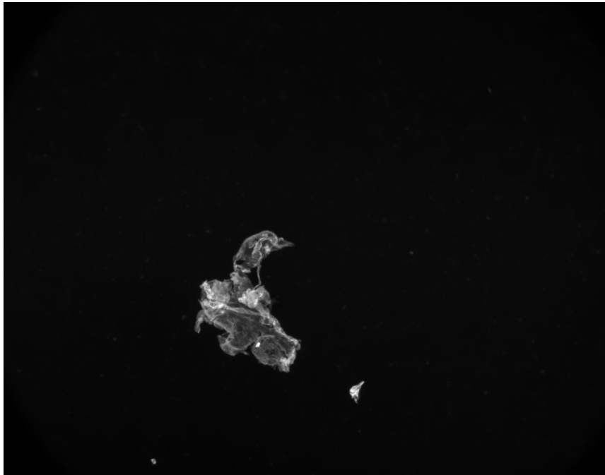
Figure 5.17 Salmonella bound to the MSCAT's surface (800x magnification)
