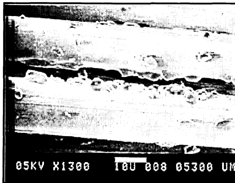
Figure 1.9. Creosote accumulation on fiber/matrix interfaces. Fibers were taken from creosote treated FRP coupons after testing.
