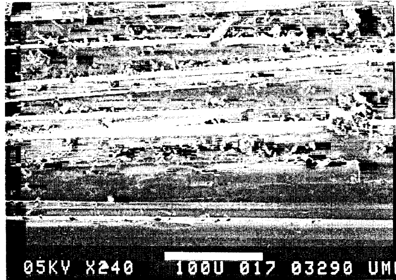
Figure 5.18 SEM Image (240X) of Hand Lay-up GFRP Tested at 40%UTS Showing Resin Debris and Fiber Fracture
