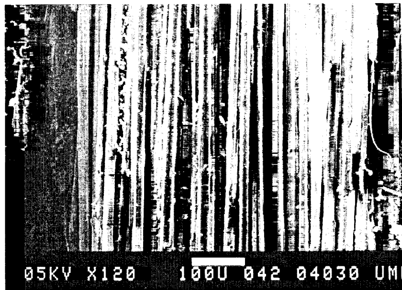
Figure 5.19 SEM Image (120X) of Hand Lay-up GFRP Tested at 40%UTS Showing Fiber Debonding and Fracture
