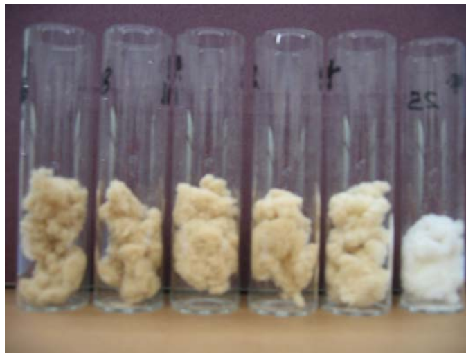
Figure D.1 Pulp Samples of Different NaOH Concentrations
