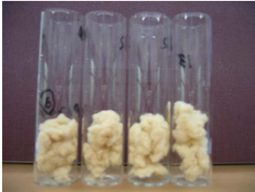
Figure D.3 Pulp Samples of Different Total Pressures
