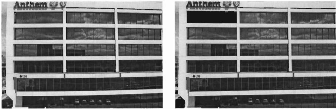
Figure 27. 24mm Lens Setting - Distortion Calibration Images Before and After Correction
