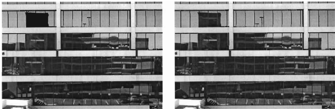
Figure 28. 35mm Lens Setting - Distortion Calibration Images Before and After Correction
