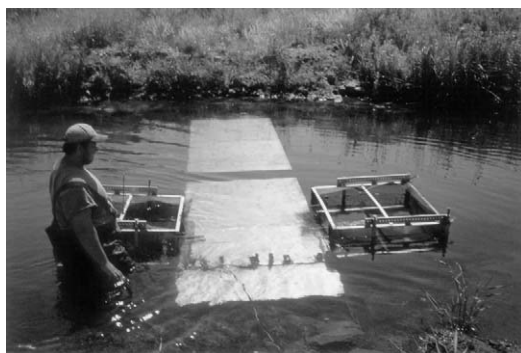
FIGURE 3.—Apparatus used to experimentally release juvenile rainbow trout over horizontal flat-plate fish screens in the field. The device is shown here attached to the Malheur fish screen. Each site required modifications to account for differences in water turbidity and the structural variations of the screens.
