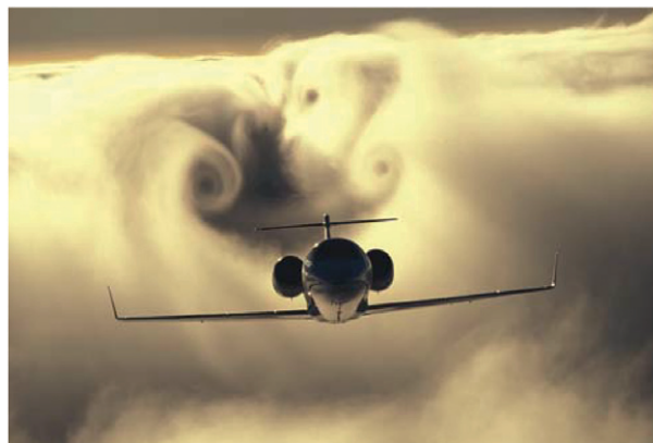
FIG. 8. Wake vortices in clouds produced by a Lear jet. Note the enhanced clustering within the vortices particularly on the left. Heavier jets produce much larger, more intense wake vortices that can extend 10 km and that are capable of disturbing precipitation-sized particles (picture by permission of Paul Bowen; available online at http://www.airtoair.net ).
